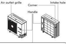
Always hold the unit by the corners, as holding it by the side intake holes on the casing may cause them to deform.
