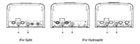
Hole A: For DC line (wire which is connected to the PCB of the control box)
