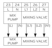
(L): Live signal from PCB to mix pump (N): Neutral signal from PCB to mix pump
