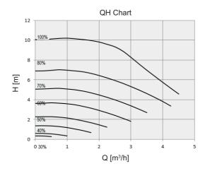
Performance test based on standard ISO 9906 with pre-pressure 2.0bar and liquid temperature 20 °C.
