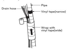
Do pipe forming by wrapping the connecting cable and refrigerant pipe (between the indoor unit and outdoor unit) with thermal insulation material and secure it with two kinds of vinyl tape.
